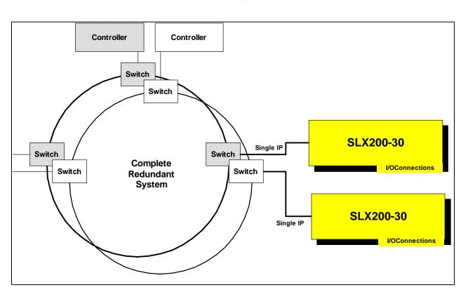
As shown in these graphics, it is no longer necessary to spend time searching for lost data as simple yet very effective methods of redundant data acquisition are readily available. Dataforth's isoLynx® SLX200-30 is a highly efficient redundant Ethernet data acquisition system that is usable across all types of redundant configurations.
