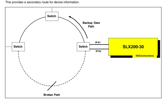
Type 3. Redundant Network Switch(es) or Node(s) These provide a secondary route for failed switches.
