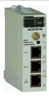
LEDs enable monitoring of LAN / WLAN activity and display the quality of the radio link in order to get the best result while installing the device.
